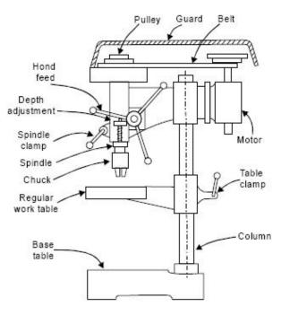
Check Belts for cracking and fraying. If a new one is needed the size is printed on the belt
