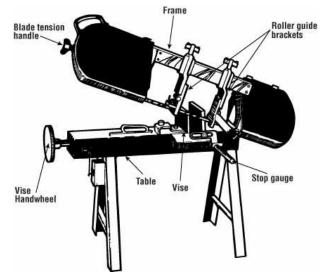
The Parts of a Bandsaw
