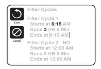
"NO" is highlighted, press Up or Down to toggle Filter Cycle 2 on and off. When Filter Cycle 2 is ON, it can be adjusted in the same manner as Filter Cycle 1 by navigating to the right. It is possible to overlap Filter Cycle 1 and Filter Cycle 2, which will shorten overall filtration by the overlap amount.
