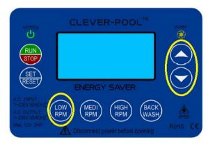
Press the RUN/STOP button to put it into run mode, this will start the pump. When the chlorinator timer turns off, the CLEVER-POOL will store the speed and resume at that speed when switched on again.
