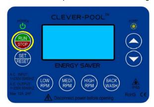
To stop the pump simply press the RUN/STOP button again.
