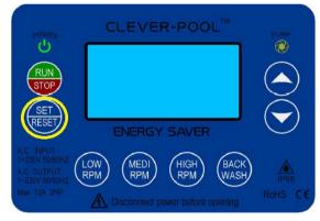
Press the SET/RESET button to step to SPEED setting. The display will now show the flashing four digits for speed, which is the speed for AUTO MODE 1. Press the up or down button to change motor speed. Alternatively press one of the systems preset speed buttons LOW RPM, MEDI RPM, HIGH RPM.
