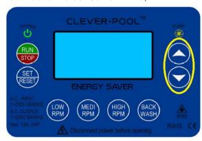
Press the SET/RESET button to step over from hours to minutes. The display will then flash the minutes digits.
