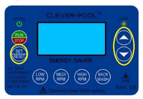
Press the SET/RESET button to store the speed and step over to AUTO MODE 2. The display should show CURRENT TIME, START TIME, STOP TIME and the stored time with hours digits flashing. This is the start time for AUTO MODE 2.
