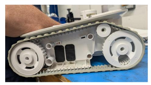
Undo the screws holding drive wheel and gears both sides. Then remove them and the track.
