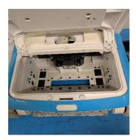
Undo the 6 clips holding the blue side cover.
