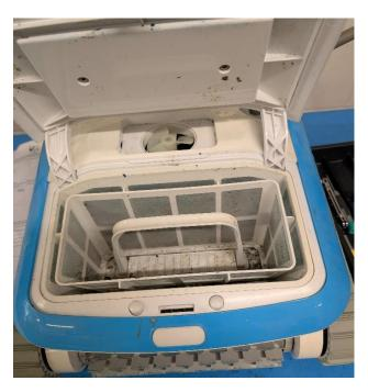
Unclip the six clips holding the Blue Trim and then remove the trim.
