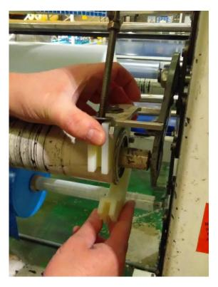
3. Close brake and tighten wing nut for required grip as per picture. Take care not to trap fingers. Avoid over tightening as this will prevent material feeding correctly.
