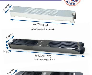
Note: The 475mm length on both single and double Stainless Steel Treads has now been replaced with 495mm length, in line with current SPATA Standards.
