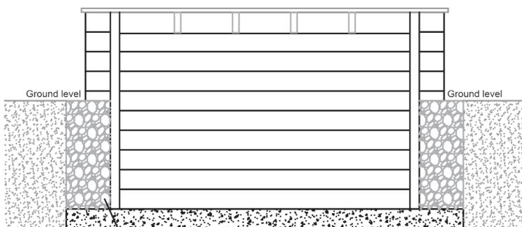
There MUST be enough back filled pea beach to allow for adequate drainage
