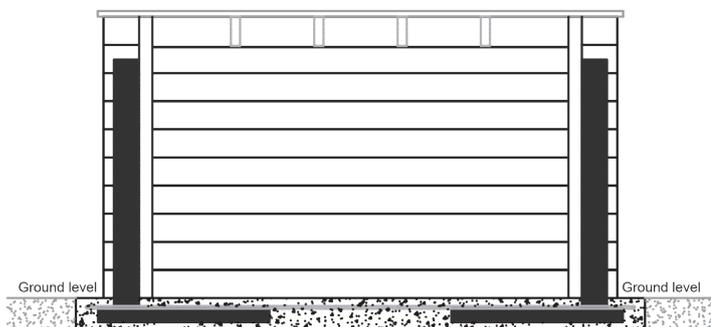
We advise a minimum of just over half of the pool is sunk before you are able to remove the braces or strap system.
