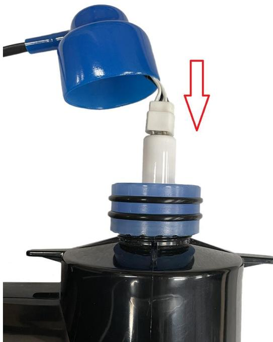
**NOTE:** Pinch the blue lamp holder shroud as you reassemble the unit to release any trapped air. Failure to release the trapped air may cause the lamp holder to disconnect from the lamp end. Turn on the water supply to check for leaks **before** reconnecting the electric supply.
