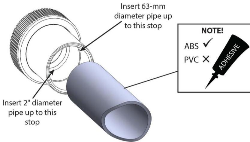
**For pipework 50-mm or 1½" in diameter.**
