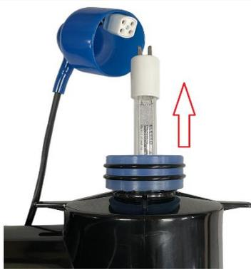
Gently slide the lamp out ensuring that no pressure is applied to the glass quartz sleeve.
