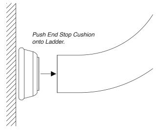
Assemble the ladder by attaching the treads to the uprights securely, using the ladder nuts and bolts provided. Then fitting the end stop cushions onto the end of the ladder.
