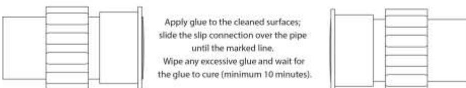
This is what the unit should look like when installed on the pipe
